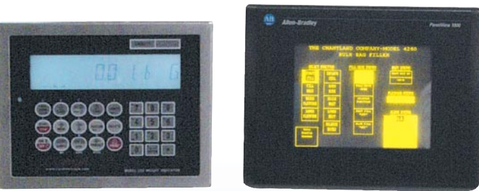
Scale Control and PLC with User Friendly Touchscreen Interface
